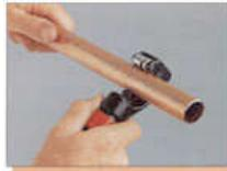
**1.** Cut the tube ends square, deburr, and if soiled or excessive oxide has built up, clean the surface with a light grade emery tape or wire brush.
