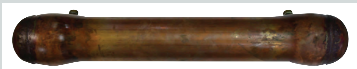
Figure 4.1b Sample after exposure to 7,500 kPa (6 times SWP)
