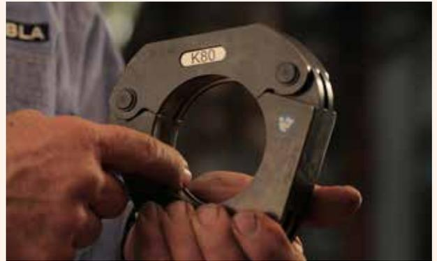
**6.** Select the appropriate sized KemPress® collar, check it is clean and that the surface of the pressing area is smooth.
