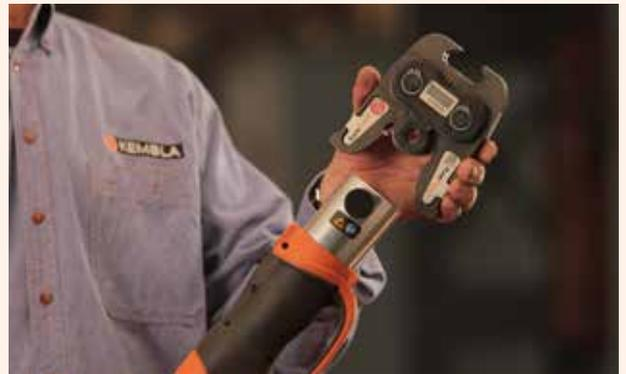
**8.** Select the ZB203 Adaptor Jaw, insert onto the KPL/ KPL2 pressing tool and arrest the locking bolts of the tool.
