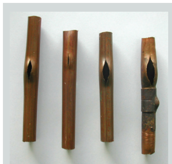
Figure 11.3 Picture Showing Pipe Burst At Subzero Temperature
