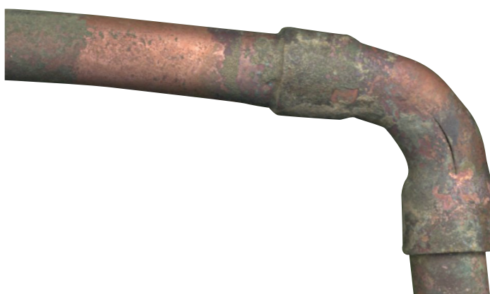
Figure 6.10 Edge Cracking due to Fatigue Corrosion of an Elbow
