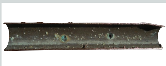
Figure 6.4 Pitting Corrosion – Warm Water Systems
