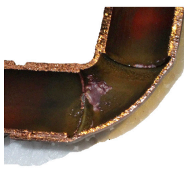
Figure 6.8 Erosion Corrosion from turbulence caused by burr left inside of tube
