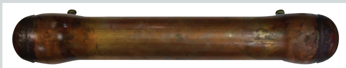
Figure 4.1b Sample after exposure to 7,500 kPa (6 times SWP)
