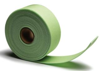
MM Kembla PipeLag is a Cross Linked Closed Cell Polyethylene lagging (XLPE) made by renowned global insulation manufacturer L'isolante K-Flex. The closed cell, tough, nonabsorbent lagging is perfect for use on drainage pipes that penetrate concrete slabs and footings.
