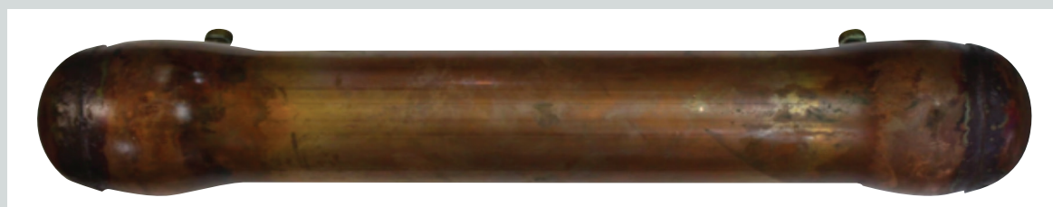
Figure 4.1b Sample after exposure to 7,500 kPa (6 times SWP)
