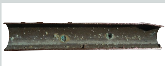
Figure 6.4 Pitting Corrosion – Warm Water Systems
