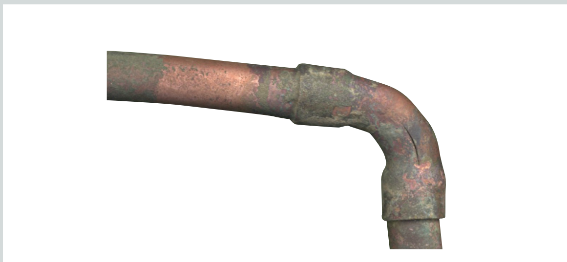
Figure 6.10 Edge Cracking due to Fatigue Corrosion of an Elbow
