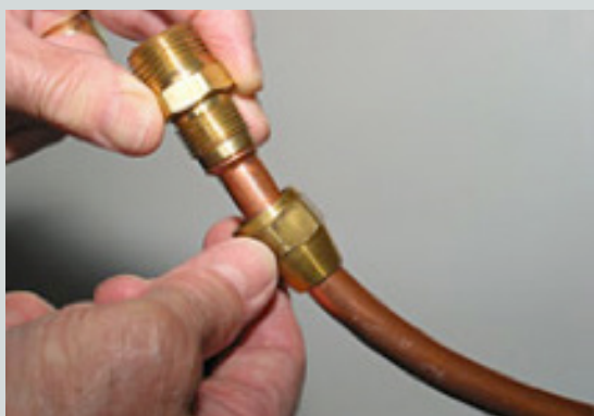
Figure 7.1a Assembling Copper Flare Pipe Adaptor and Nut
