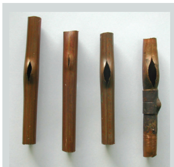
Figure 11.3 Picture Showing Pipe Burst At Subzero Temperature
