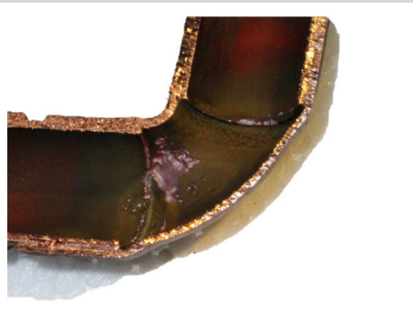
Figure 6.8 Erosion Corrosion from turbulence caused by burr left inside of tube
