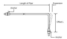
Table 2 shows the length of the offset required for various diameter copper tubes based on the expansion estimated from Table 1.
