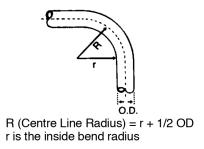
The following formula, which takes into account the tube's ductility, may be used as a rough guide for determining minimum bend radii:
