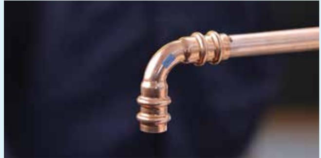
**8.** Slide the fitting all the way up to the insertion depth mark and until you make contact with the fittings stop. It is critical that full insertion depth has been achieved before pressing.
