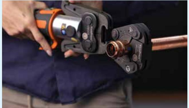
**14.** Attach the ZB203 Adaptor Jaw onto your KemPress KPL3 press tool and lock it by engaging the locking pin. Open the adaptor jaw and attach it to the pins on the Streamline ACR Press Collar.
