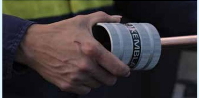
**2.** Deburr the end of the tube on the inside and outside to minimise turbulence and pressure loss, and to avoid damaging the fittings O-rings. A conical deburrer is recommended to deburr the outside diameter, and a conical deburrer or pin reamer may be used for the inside diameter.
