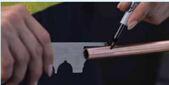
**5.** Mark the fitting insertion depth on the tube with a Streamline ACR press gauge tool. Whilst this is the preferred method, you can also use a tape measure and reference the insertion depth chart on the back of the bag.
