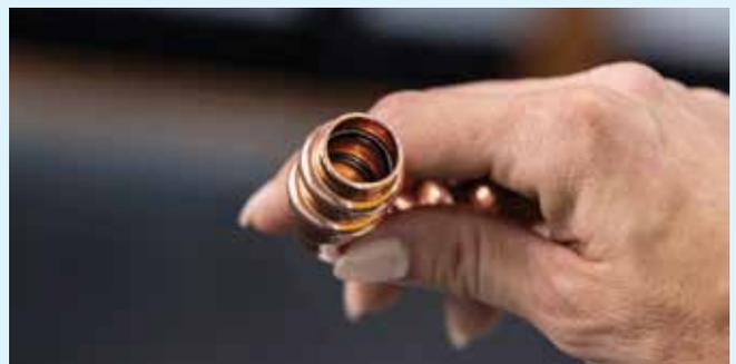
**6.** Select the correct size fitting and check both ends of the fitting to ensure two seals are present either end and correctly seated in position. Also ensure the fitting is free from of any dirt or debris before using. It is recommended the fittings are stored in their resealable bags prior to use, to prevent contamination.
