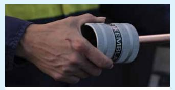
**2.** Debur the end of the tube on the inside and outside to minimise turbulence and pressure loss, and to avoid damaging the fittings O-rings. A conical deburrer is recommended to debur the outside diameter, and a conical deburrer or pin reamer may be used for the inside diameter.
