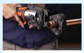
**14.** Attach the ZB203 Adaptor Jaw onto your KemPress KPL3 press tool and lock it by engaging the locking pin. Open the adaptor jaw and attach it to the pins on the Streamline ACR Press Collar.
