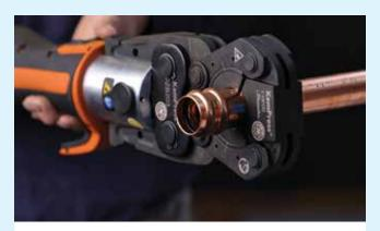
**15.** Check the fitting is still fully engaged to the insertion depth mark and once the jaw and fitting is correctly engaged, initiate the pressing process by holding down the start button.
