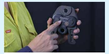
**9.** Select the correct size Streamline ACR Press Jaw and check the jaw is in good condition and its press surface is clean and free from debris.
