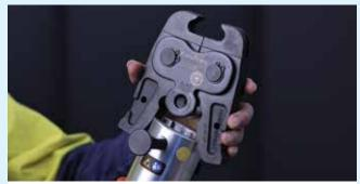
**12.** For fittings sizes inch and one eight and greater, use the ZB203 Adaptor Jaw and corresponding size Streamline ACR Press Collar.
