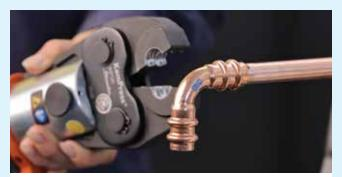
**10.** Attach the jaws onto your KemPress KPL3 tool or other compatible full size 32 Kilo Newton press tool and lock it by engaging the locking pin. If using a KemPress KPS2 press tool, ensure you use Streamline ACR Press small jaws, as large and small tool jaws are not interchangeable.
